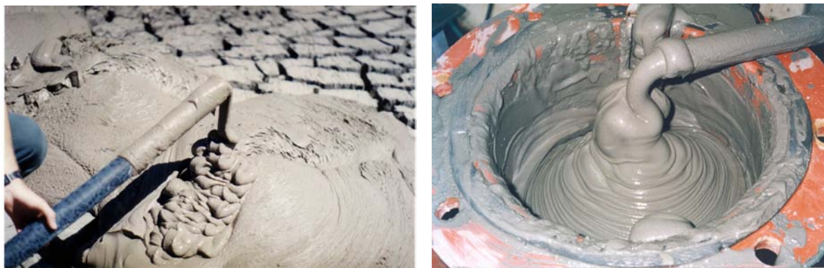
Figure 1.3 Examples of Ultra High-Density (Paste) Thickened Tailings
